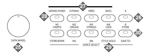
**25 DATA WHEEL:** Use the data wheel to quickly scroll through available selections or options within the pianos features and functions.
