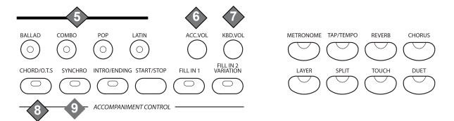
**5 QUICK SELECT STYLE BUTTONS:** There are four Rhythm Styles that can be selected quickly by pressing one of the four quick select rhythm style buttons. The rhythm style name is printed above the style select button. Press a button to select the style of your choice. The selected rhythm name and its number will be shown on the display.
