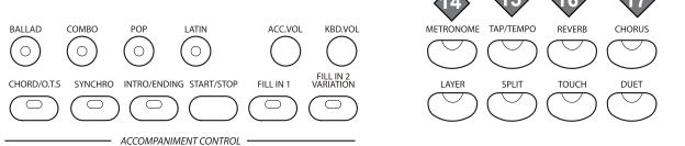
**14 METRONOME:** The metronome is a convenient feature for practice, and can also provide a solid rhythmic guide when recording. The METRONOME button toggles the metronome feature on and off. Press the metronome button to hear the tempo & beat.
