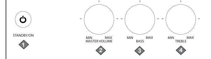
**1 STANDBY: /ON** The power switch is located to the left of the keys. Press the button to turn the power on and off. The LCD screen, and the indicator lights for the start up settings, will light up when the power is turned on.
