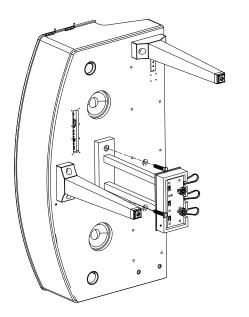
3. Attach Lyre supports to the lyre and piano body as shown. Use two lyre screws at each point shown.
