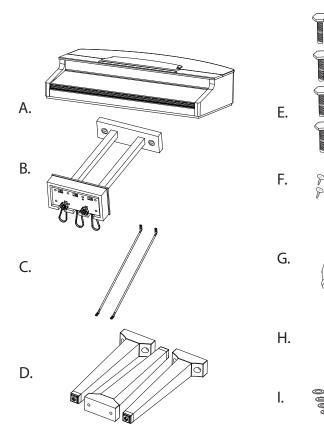
A. Piano Body B. Lyre C. Lyre Support Rods x 2 D. Legs x 3 E. Leg and Lyre bolts F. Lyre Support Rod Screws x 8
